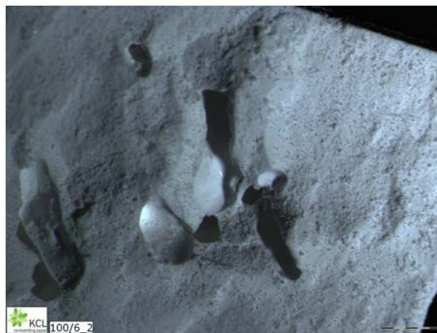
Fig. 3 Optical microscope image of part of the tablet structure (ngcc 6 pph latex) prior to grinding (the scale bar on the bottom right represents 1 mm)
